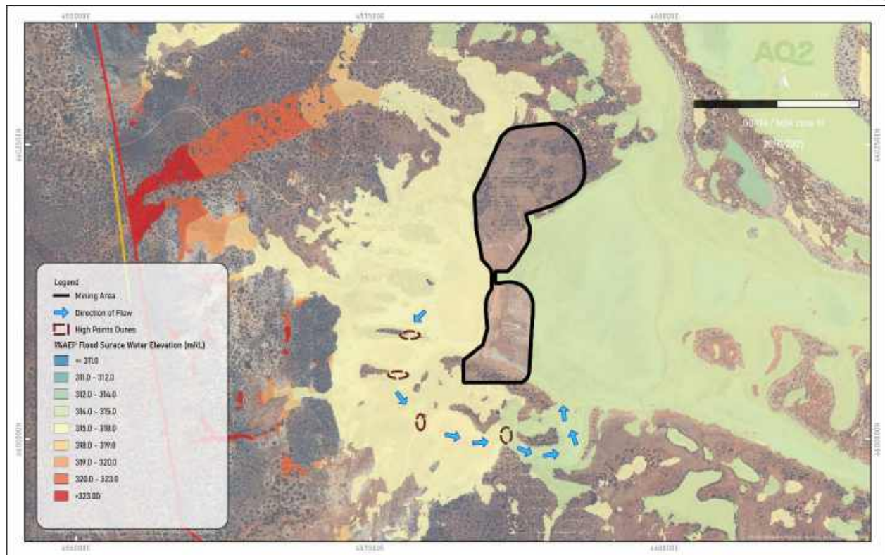
Figure 5.3 Runoff Draining Around the Mining Area
