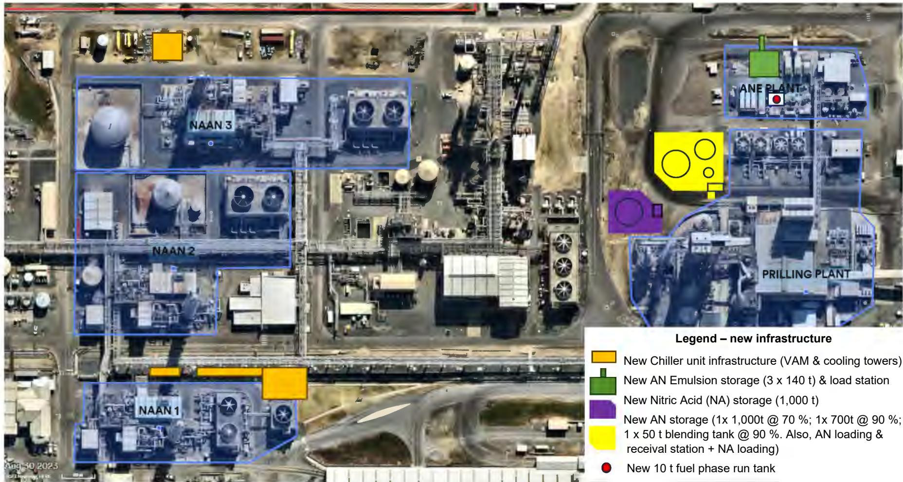
Figure 5: Indicative location of existing and proposed nitric acid and ammonium nitrate infrastructure at CSBP Kwinana associated with this application.
