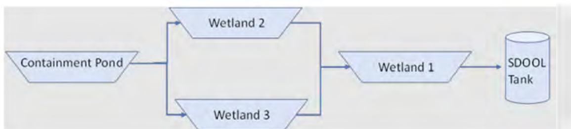
Figure 28: Wastewater treatment system
