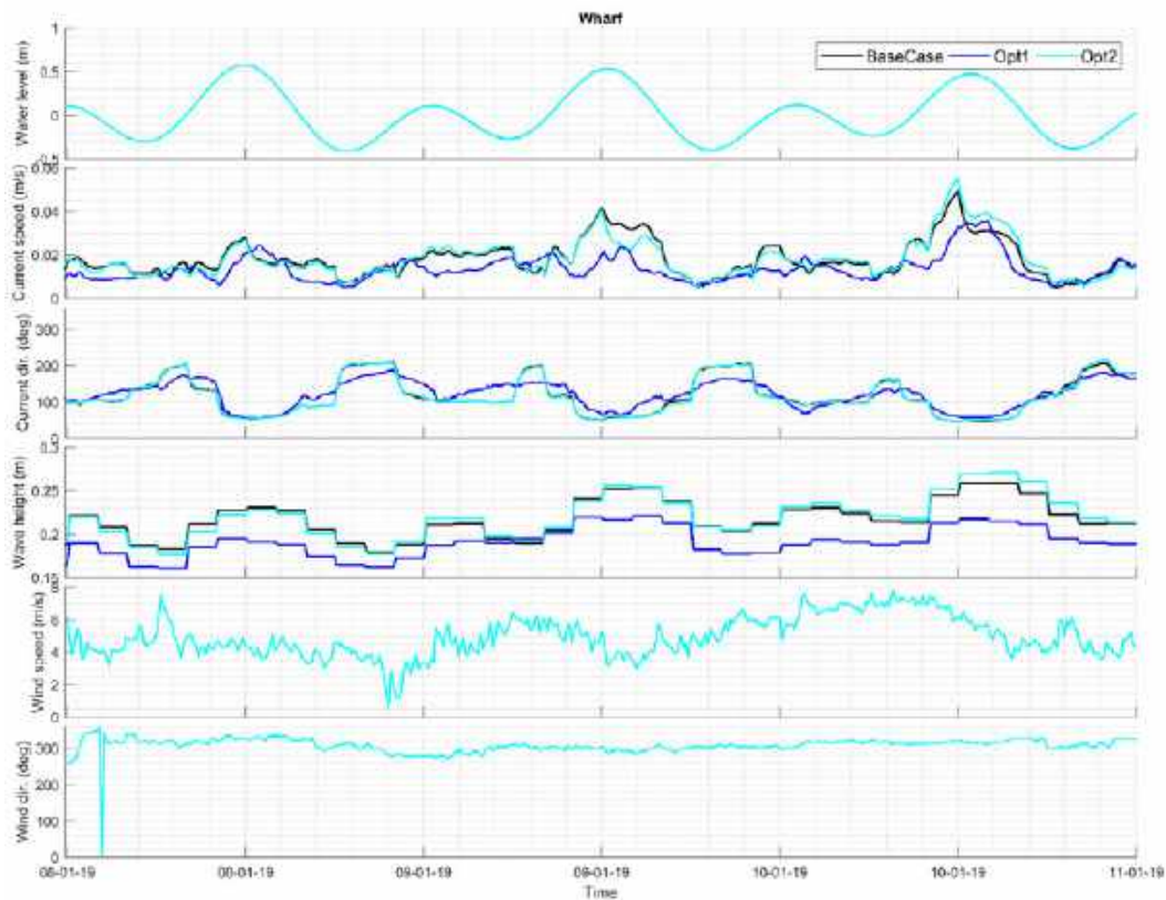
Figure 22: Comparisons of water levels, current speeds and direction, wave heights and winds at the wharf output location over the three model setups of base case, solid MOF design (solid) and piled MOF design during a period with low-energy wave conditions on 5 th January 2019
