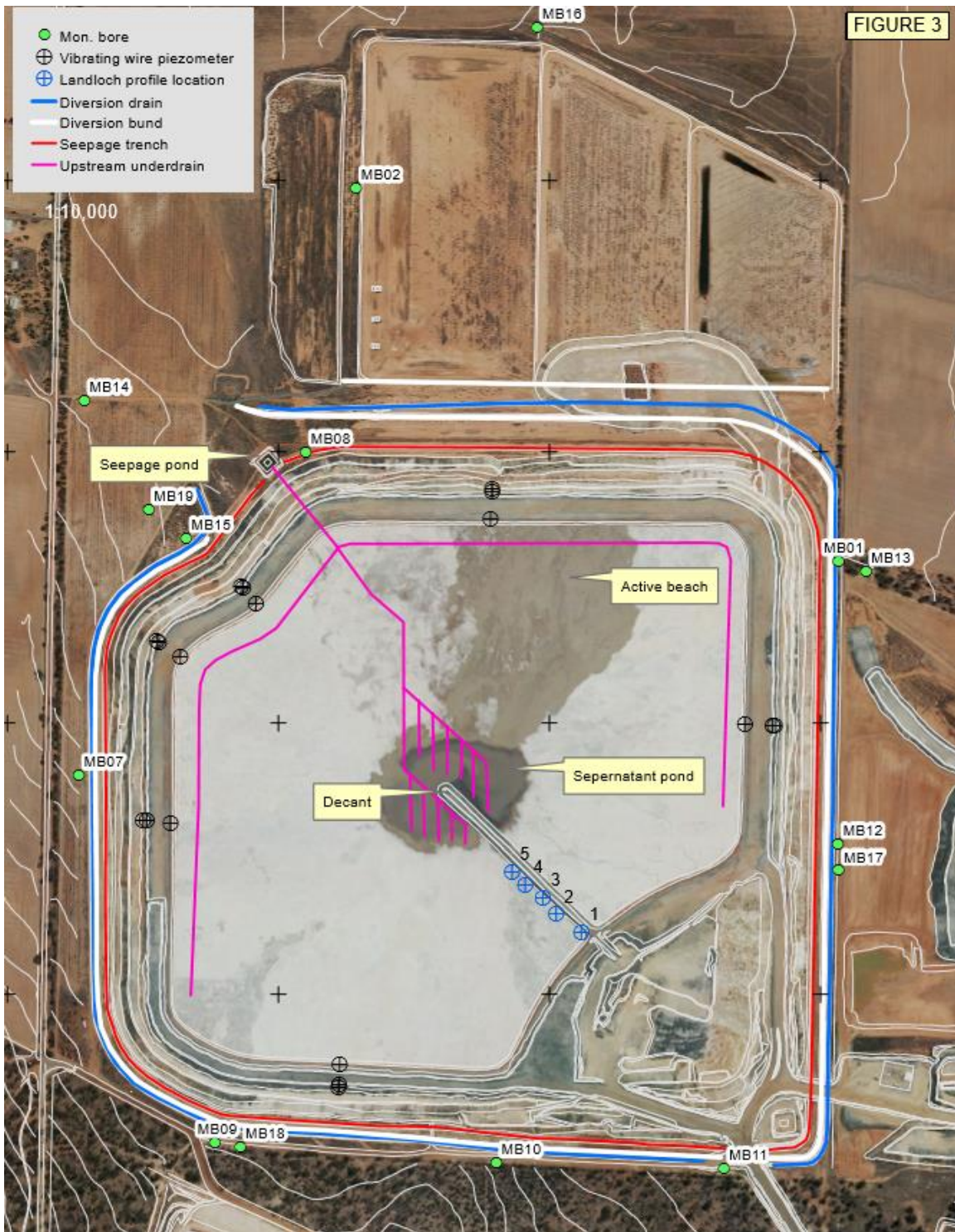
Figure 2 IWL/TSF drainage system and monitoring bores
