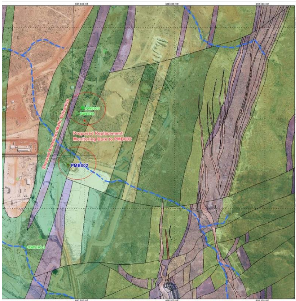
Figure 4: Location of PMB002 and proposed monitoring bore PWE033, overlaid with geological formations.
