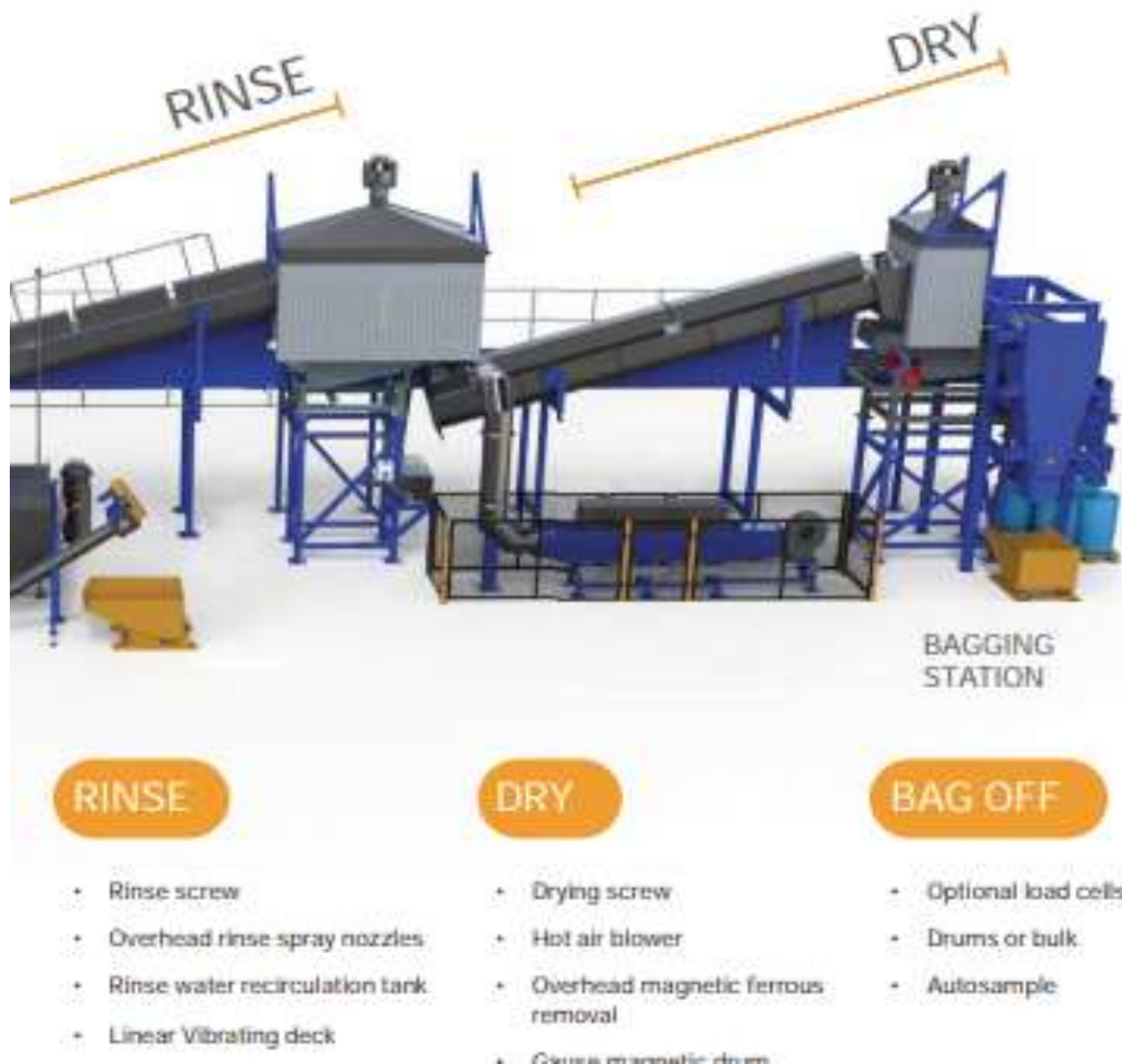
Figure 1: Basic structure of the Rotajet swarf washing line
