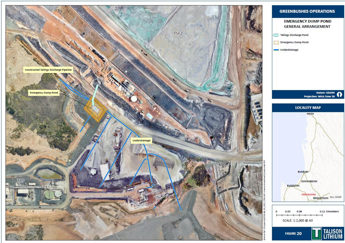
Figure 3: Location of the Emergency Dump Pond, including detail of the installed underdrainage
