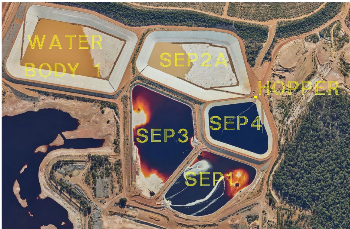
Figure 2: SEP 2A in relation to SEPs 1-4 and Water Body 1 and the hopper used to supply oxalate to SEP 2A.
