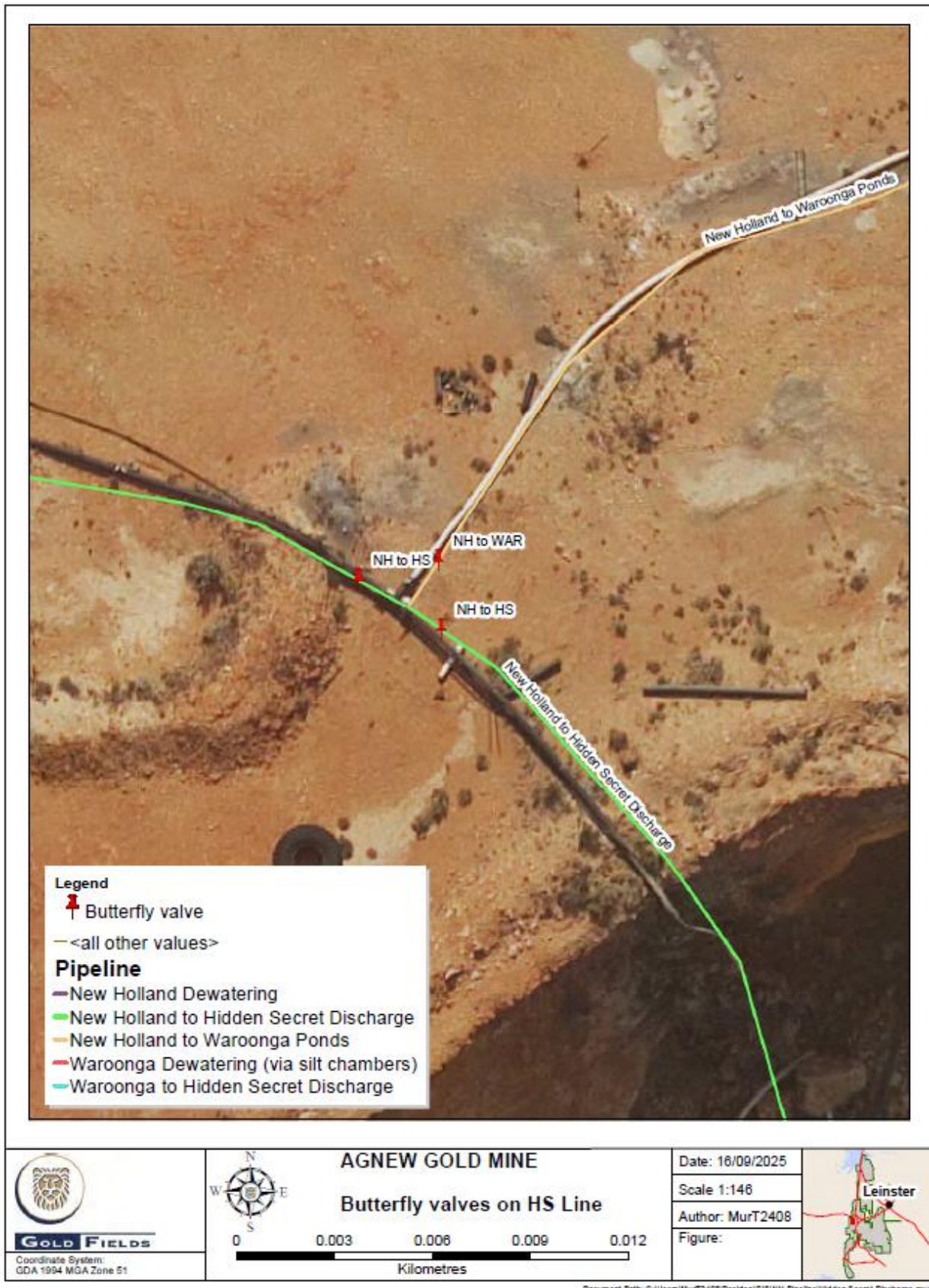
Figure 6: New Holland to Hidden Secret pipeline modification to allow discharge to Waroonga Ponds
