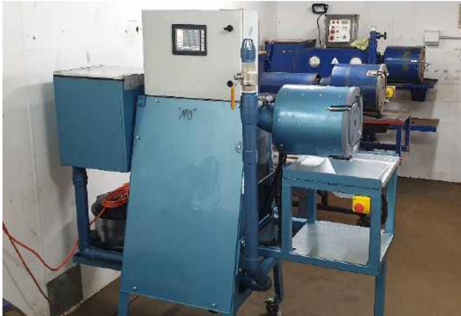
Figure 1 Dust extinction moisture test rig.
