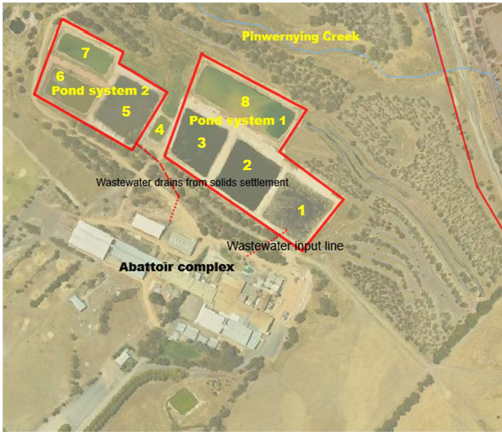
Figure 1: WAMMCO Katanning abattoir complex and wastewater ponds
