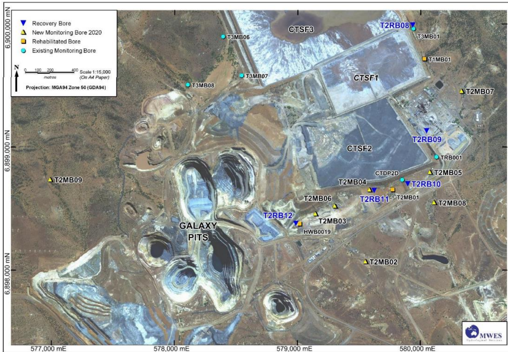
Figure 1 Groundwater monitoring bores and seepage recovery bores proposed for addition to licence
