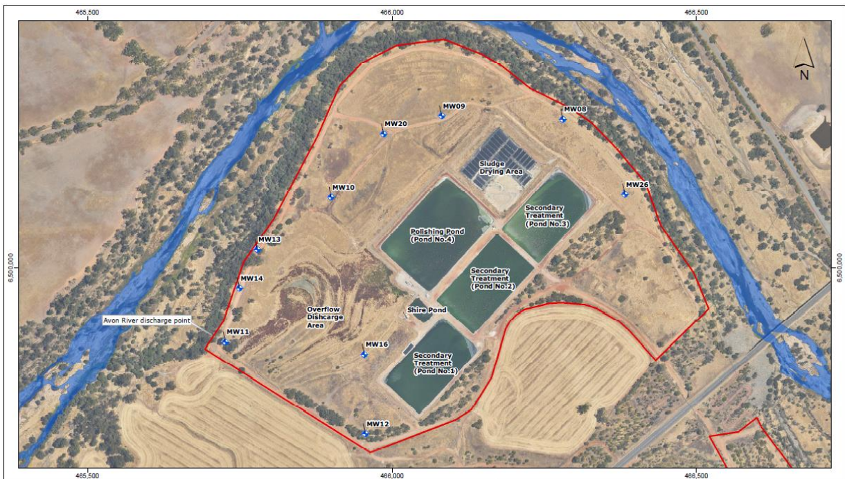
Figure 7: Groundwater monitoring bore locations
