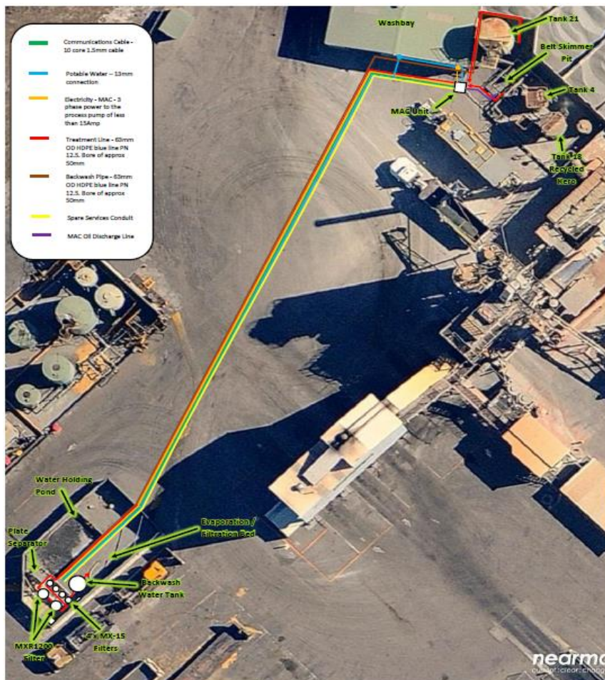
Figure 1: proposed washbay wastewater treatment upgrades layout.
