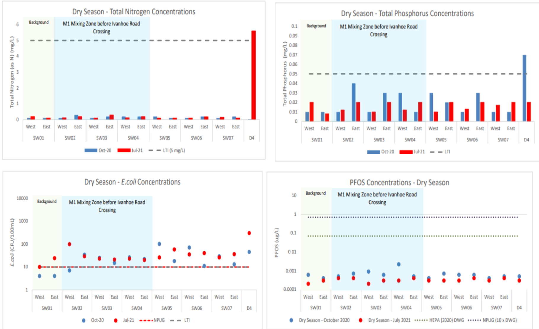
Figure 5: Dry Season irrigation period TN, TP, E. coli and PFOS concentrations relative to applicable EIL
