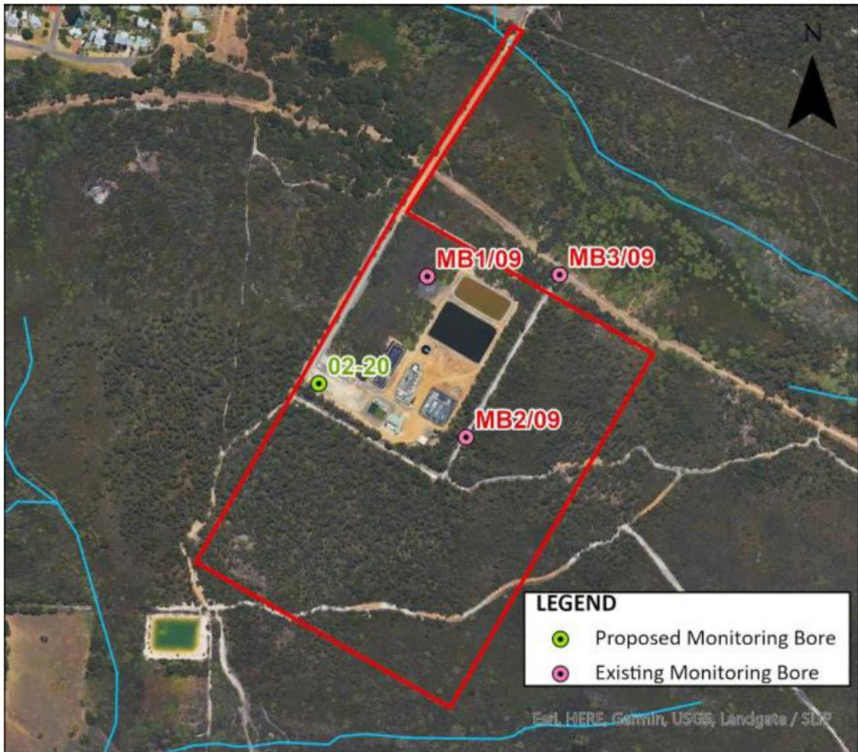
Figure 1: Existing and proposed monitoring bores
