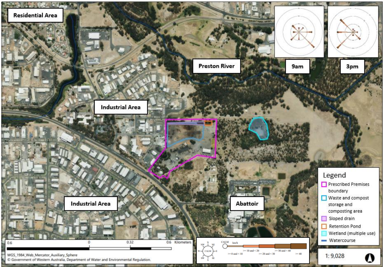
Figure 1: Prescribed premises receptor map showing average annual prevailing wind (wind roses source: BoM Station 009965)
