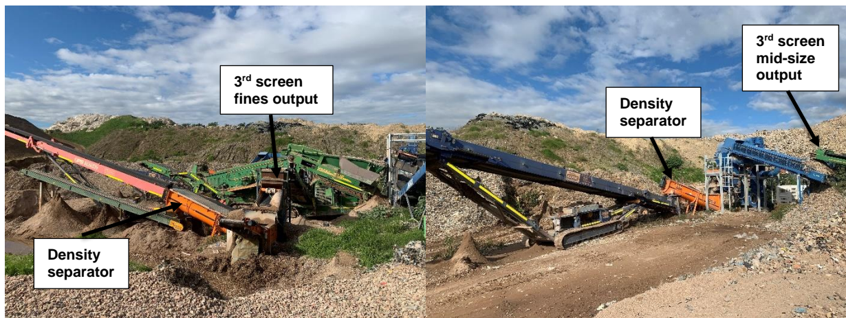
Figure 6: Fines density separator (left). Mid-size density separator (right)
