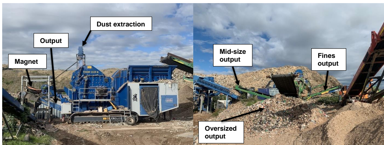
Figure 5: Hammermill shredder (left). 3 rd screen and outputs (right)
