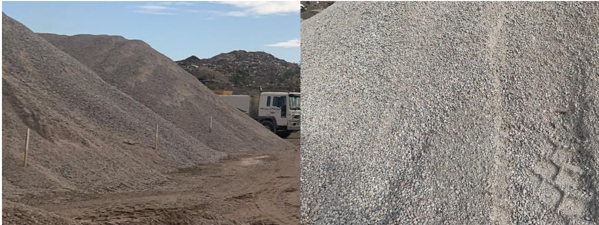
Figure 10: Recycled output stockpiles (left). Road-base output (right)
