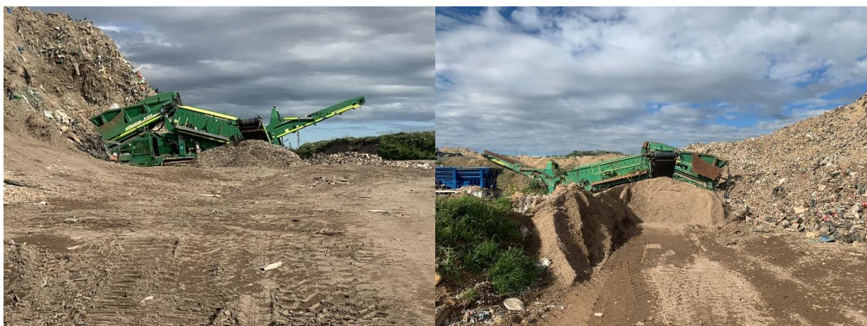
Figure 4: 1 st screen and outputs (left). 2 nd screen and fines output (right)
