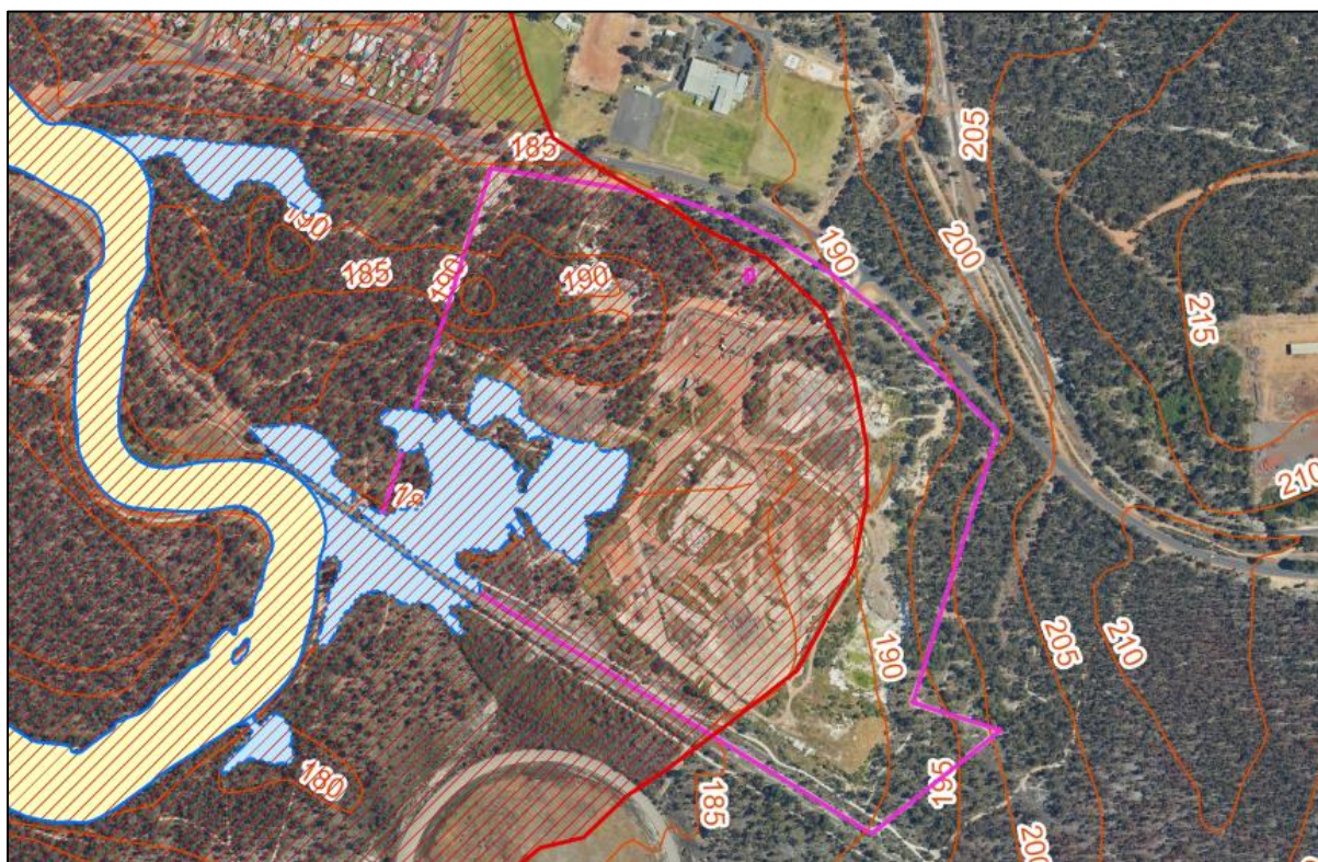
Figure 7: 1 in 100 (1%) AEP floodway (yellow area) and fringe (blue area) and floodplain development control area (red hashed area)
