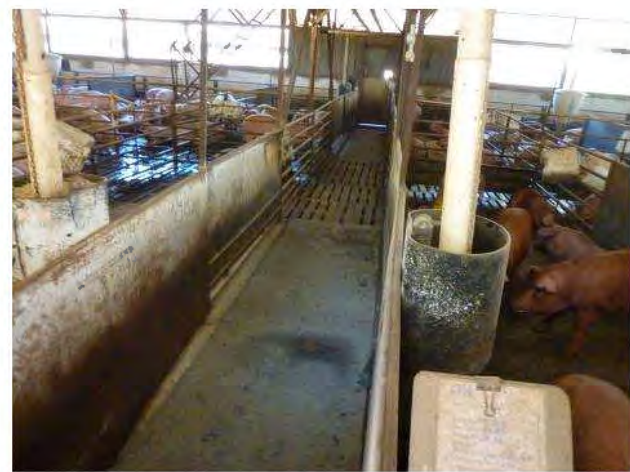
Photo 3 – Conventional shed showing slatted floors for drainage
