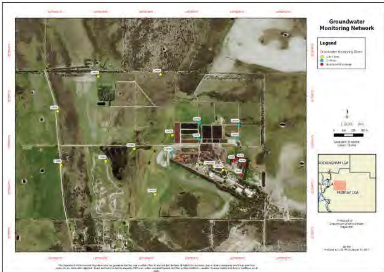
Figure 1: Groundwater monitoring bore network for CM Farms, C-Wise and Mushroom Exchange
