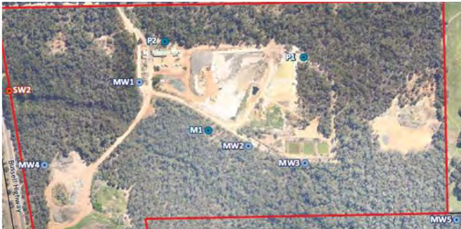
Figure 2: Location of existing groundwater monitoring bores on the Premises (excerpt from the Application)
