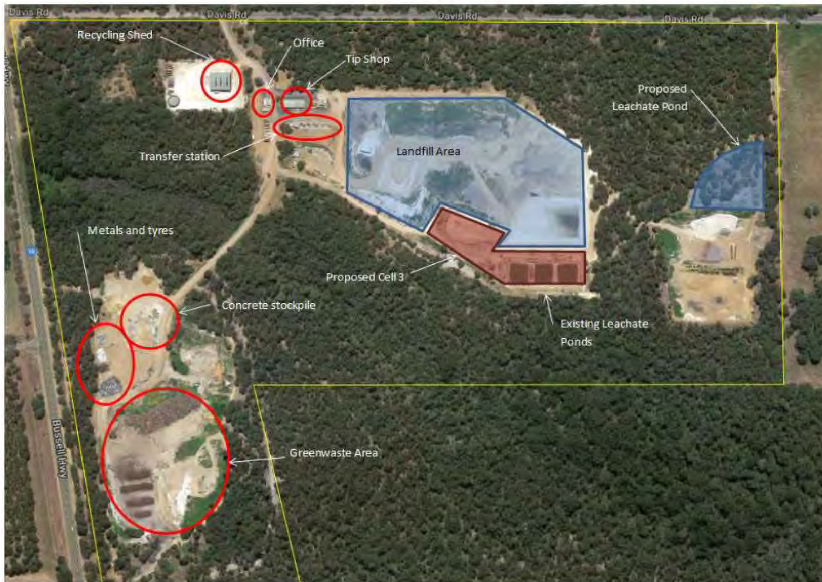
Figure 1: Site Layout Plan including proposed Cell 3 and new leachate pond (excerpt from the Application)
