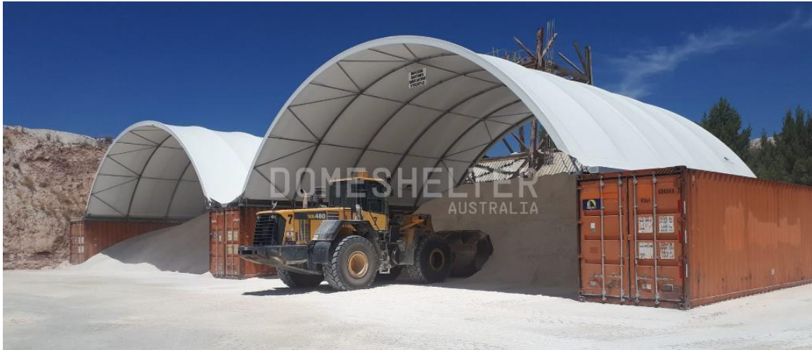
Figure 4 Example roof structure (Source: DomeShelter)
