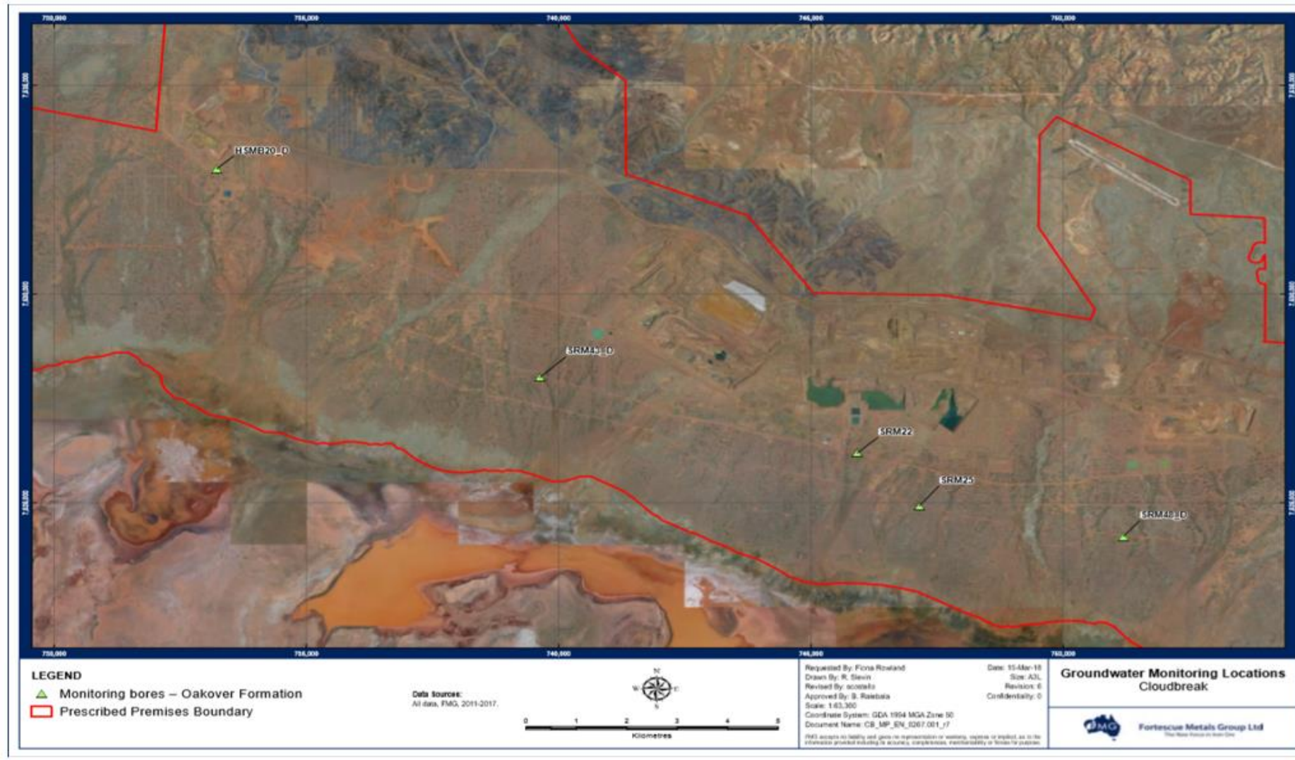
Figure 8 Licence L8199/2007/2 groundwater monitoring points (mine dewater reinjection)
