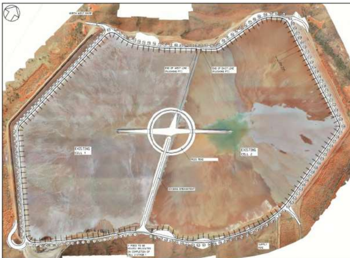
Figure 2: TSF2 single cell design, rock ring and spigots location
