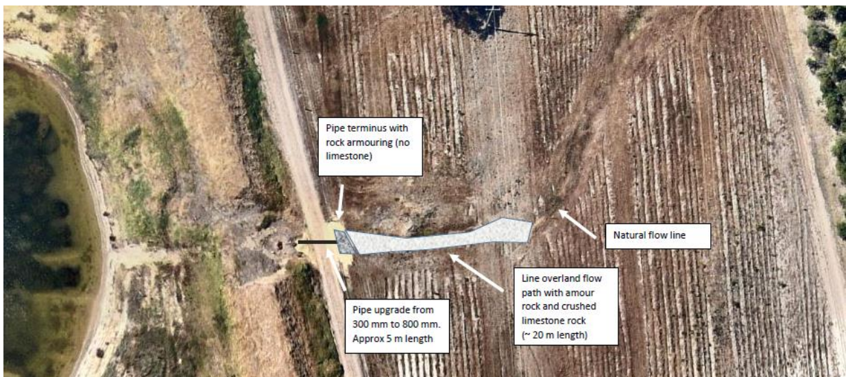
Figure 2: Upgrades to discharge point W2
