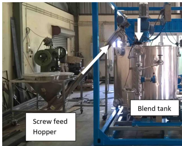
Figure 4 Screw feed hopper location
