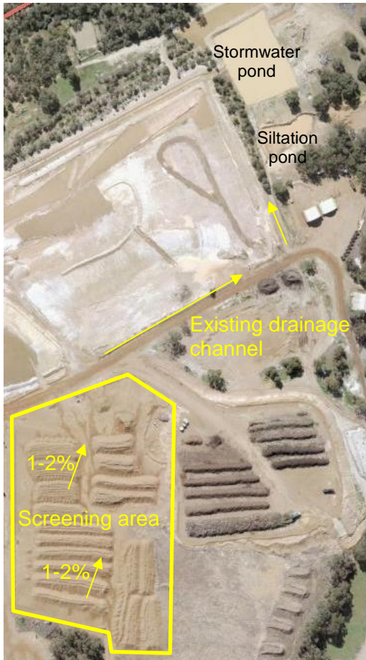
Figure 9: Current screening area and related stormwater infrastructure near Stage 14 cell
