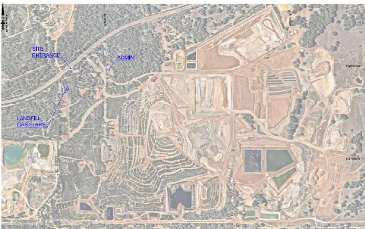
Figure 2: Proposed landfill gas flare location
