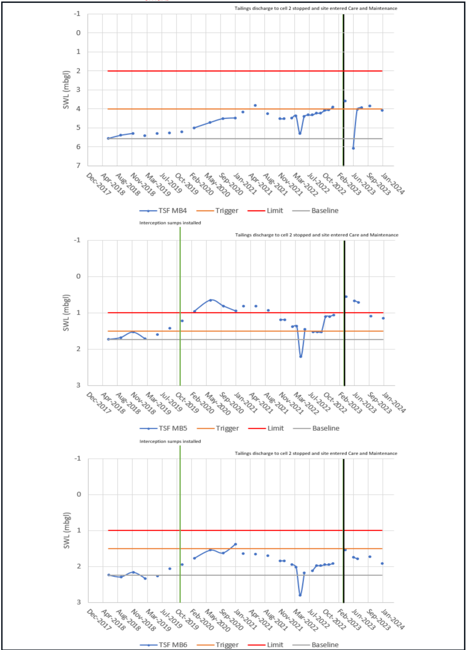
Figure 5: Historical groundwater levels with baseline, trigger and limit levels for TSF Cell 2 trigger and action values sourced from GRM 2021
