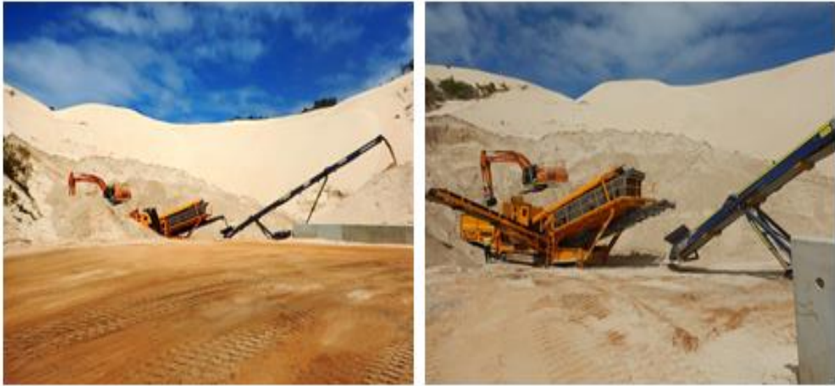
Figure 3: Screening operation conducted on M70/1302 during DMIRS site inspection.
