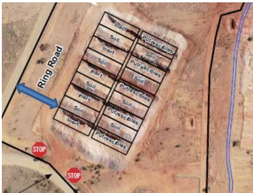
Figure 13: Landfill Trenches Layout
