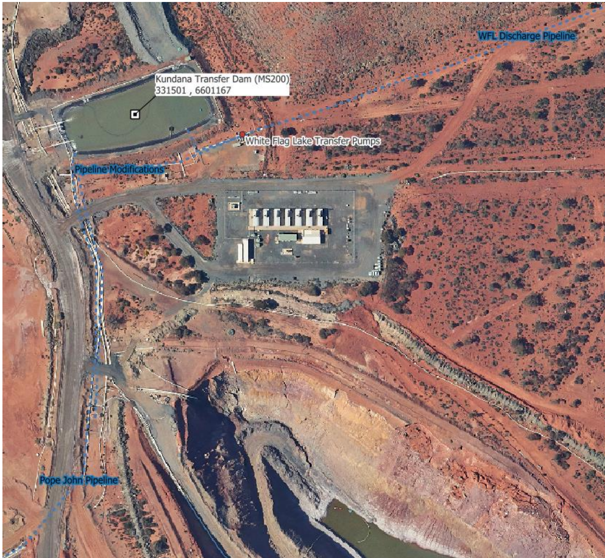
Figure 1: Pipeline modifications between Pope John Pipeline to the White Flag Lake transfer pumps
