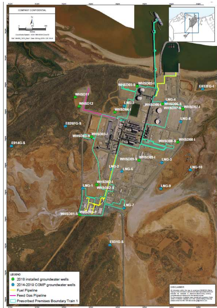
Figure 9 Wheatstone Foundation Project existing monitoring well network (Chevron)
