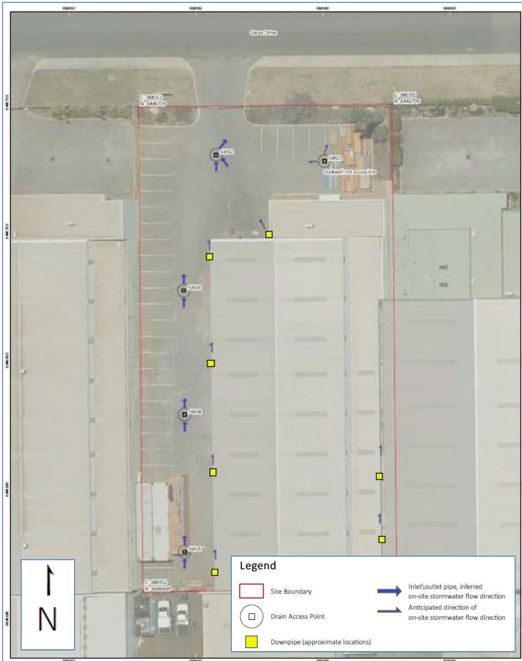
Figure 3: Premises drainage map
