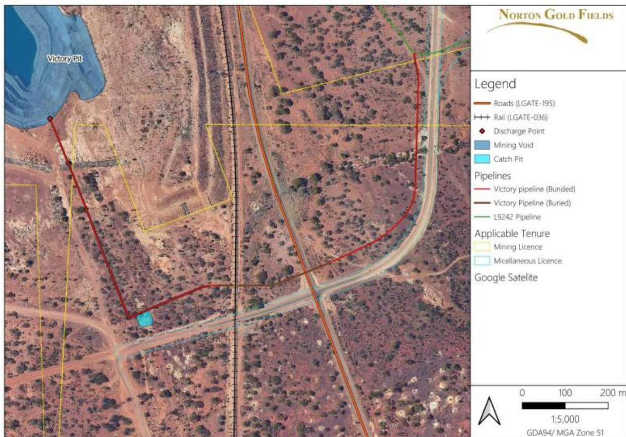
Figure 1. Victory pipeline route
