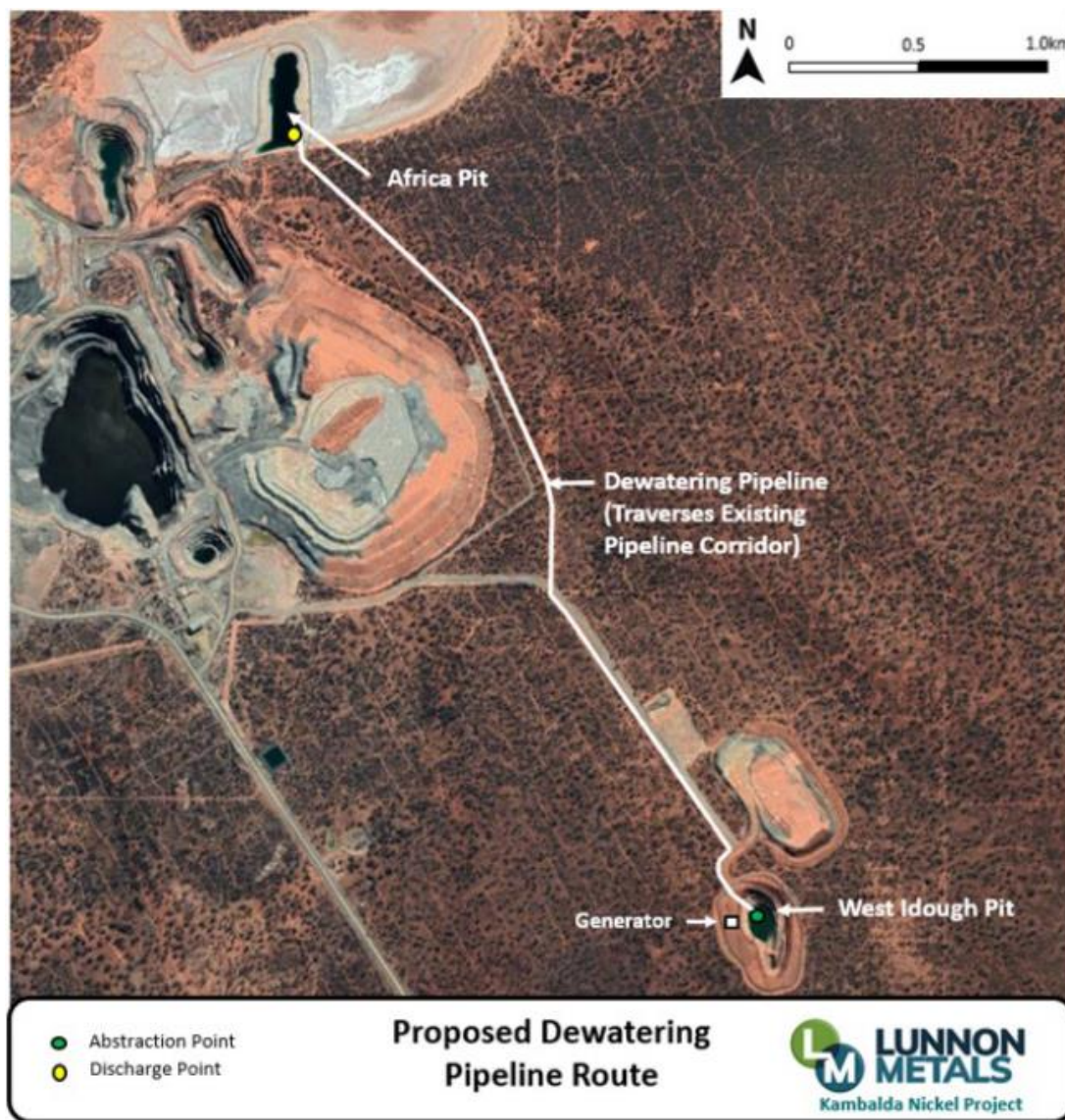
Figure 8: Proposed dewatering pipeline route.
