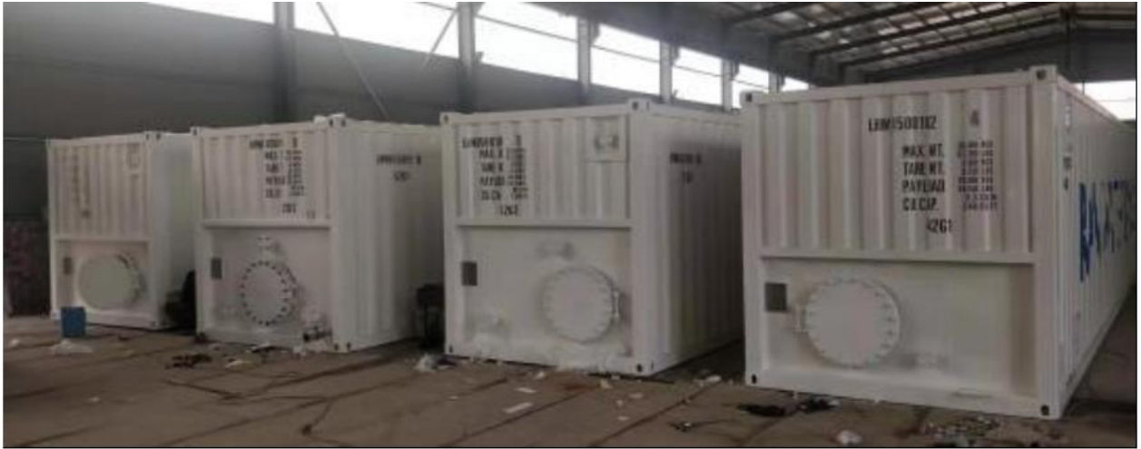
Figure 9: An example of sea container sediment settlement
