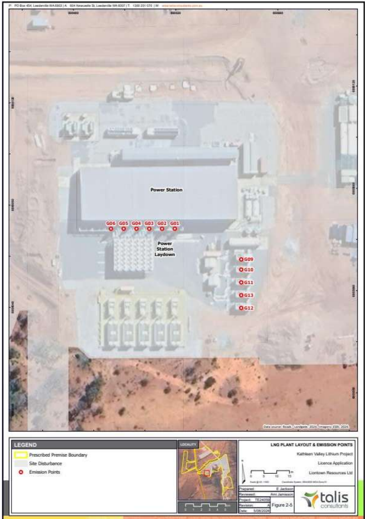
Figure 6: LNG power station emission points
