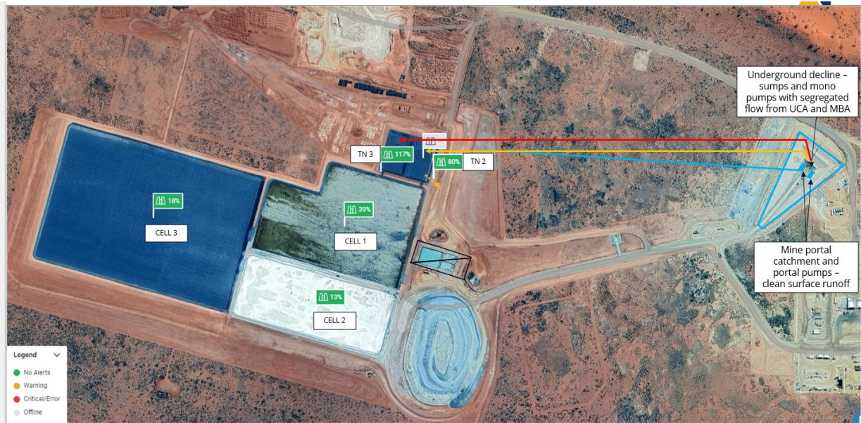
Figure 1: Dewatering system flow diagram
