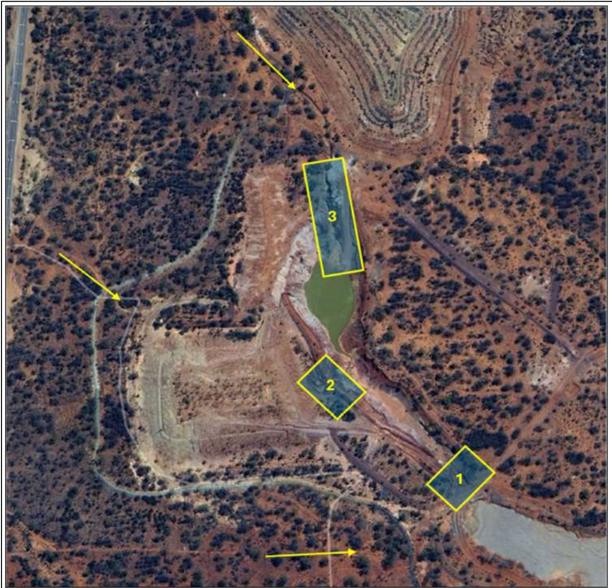
Figure 3: Graveyard in-pit TSF proposed tailing discharge locations
