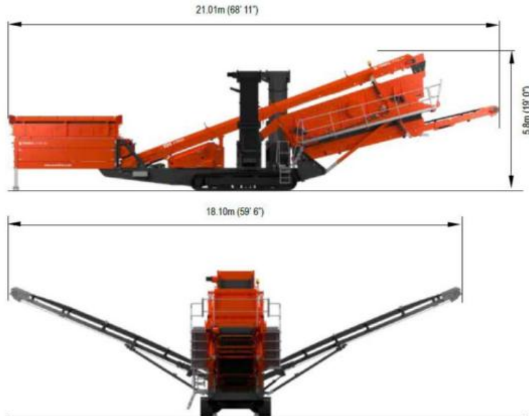
Figure 4: Working Dimensions of 696 inclined screen
