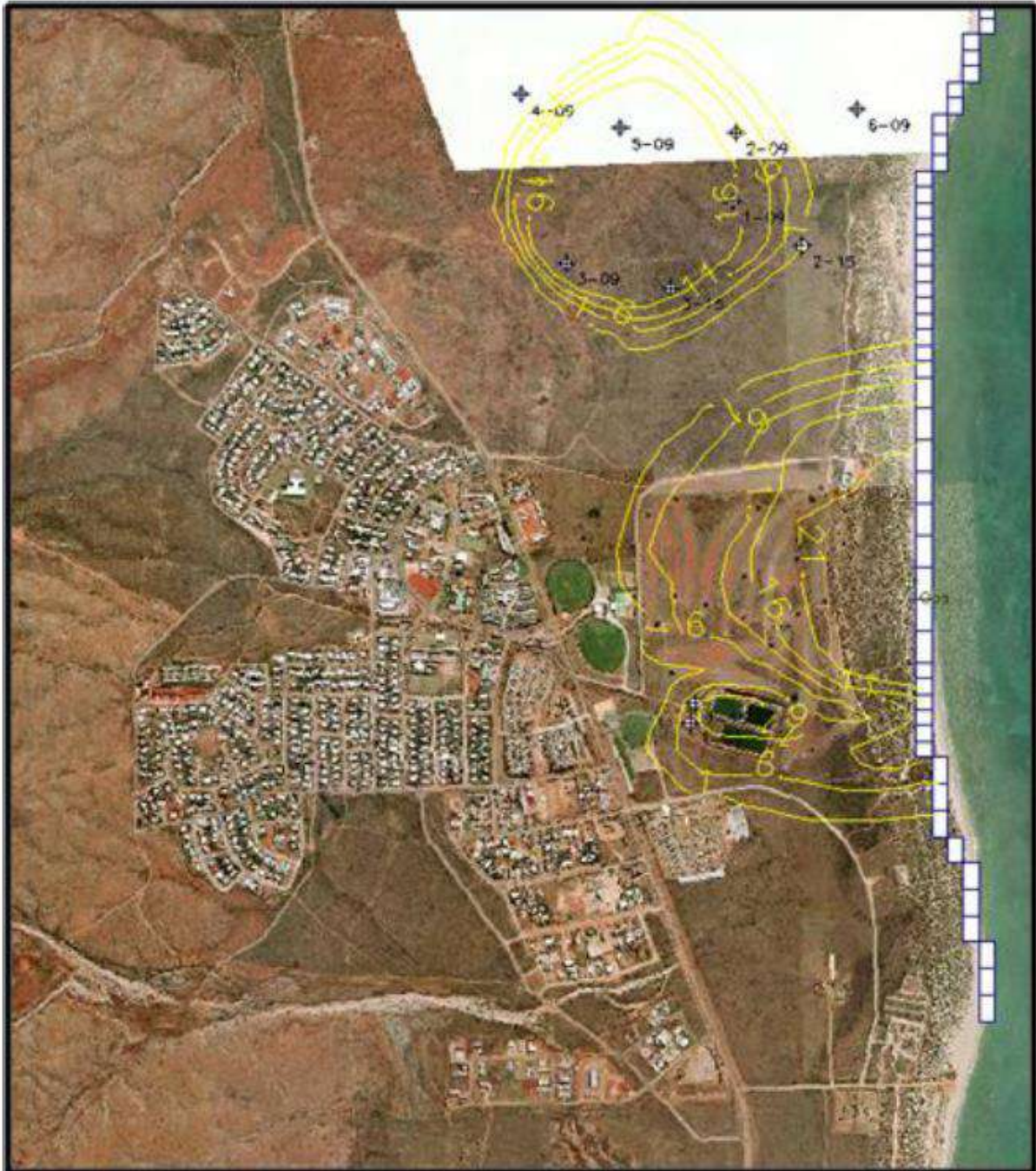
Figure 5 Modelled groundwater TN Infiltration concentrations
