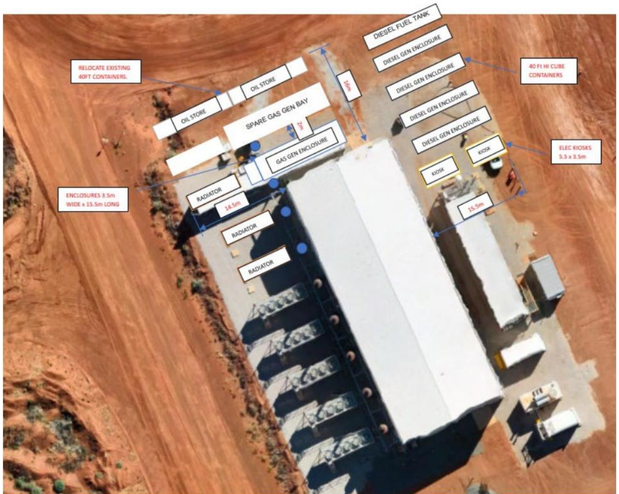
Figure 1: Power station upgrade layout ( Source: SO4 ).
