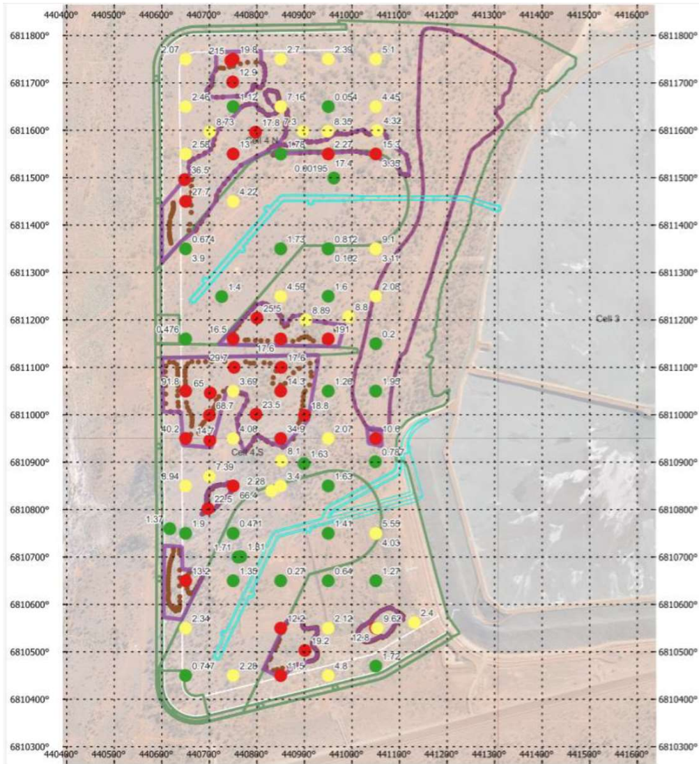
Figure 13: In situ permeability tests 2023 with TSF 2 tailings/Childe Harold Waste dump
