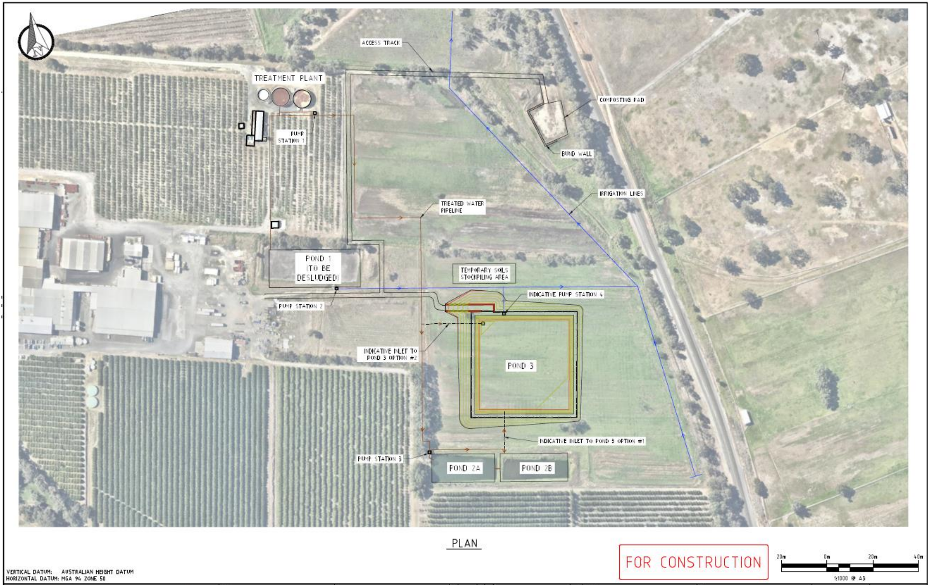
Figure 1: Proposed location of Pond 3, including indicative pump station location, and location of Pond 1, to be desludged.
