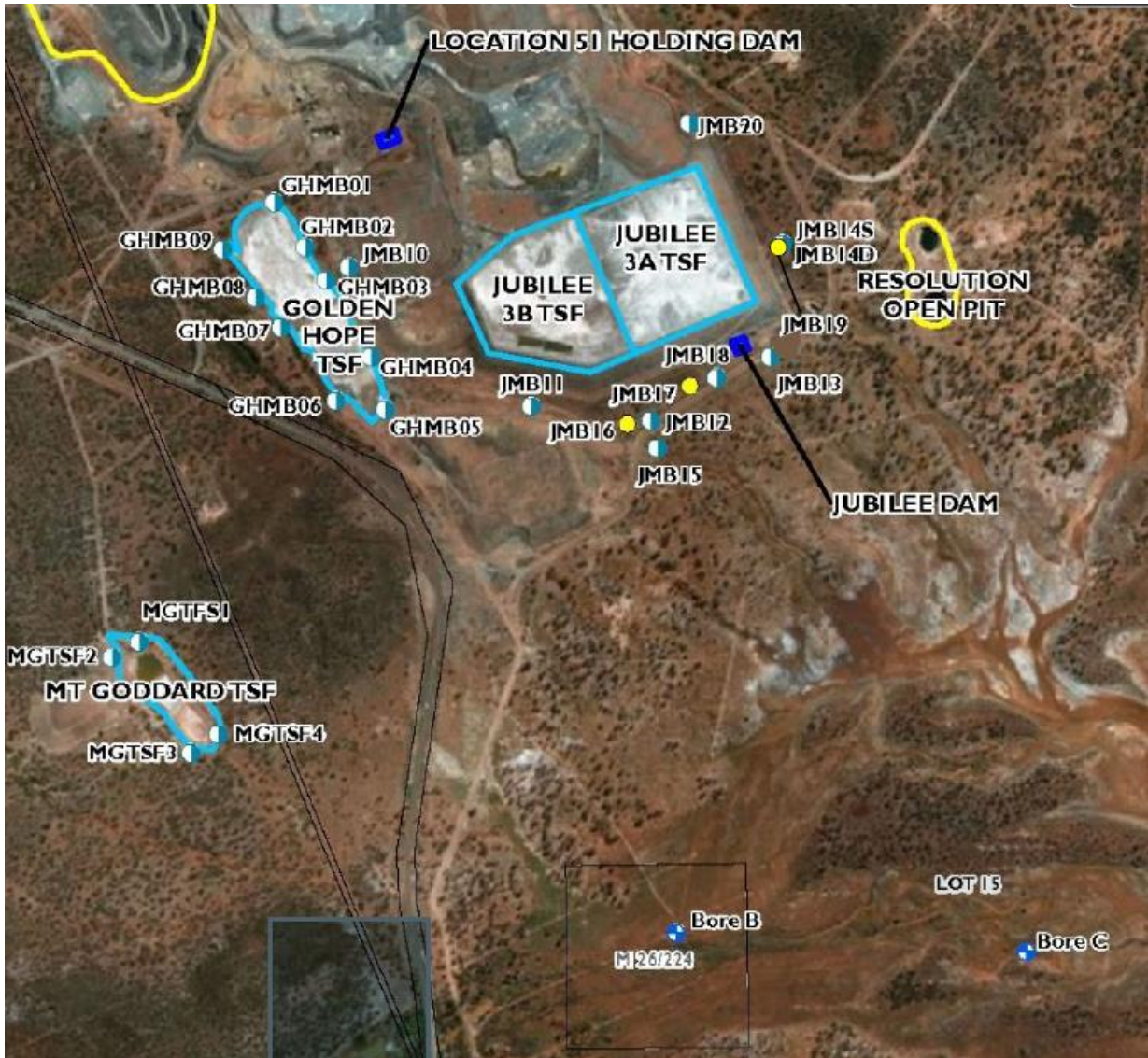
Figure 4 Existing production bores Bore B and Bore C south of TSF3A/3B.
