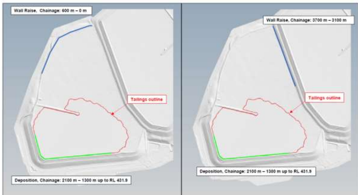
Figure 3: Cell 3 construction stage 1 (left) and 2 (right)
