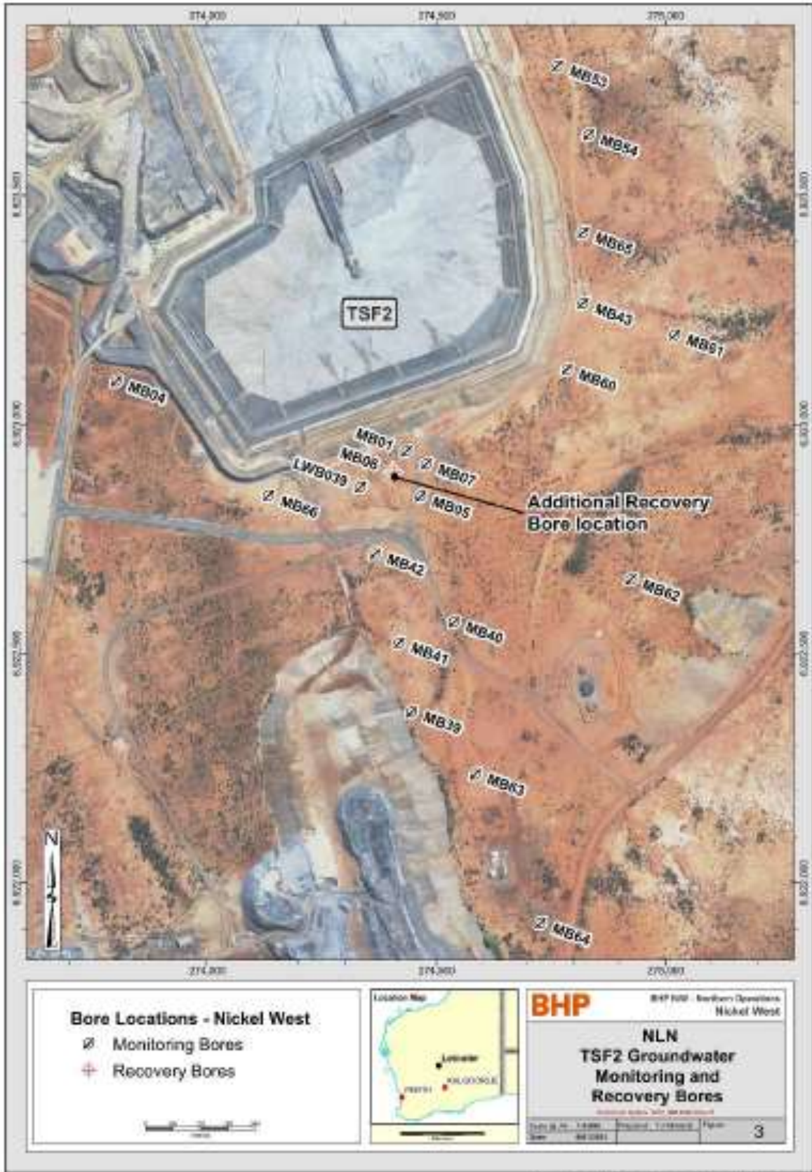
Figure 4: Groundwater monitoring and recovery bores surrounding TSF2
