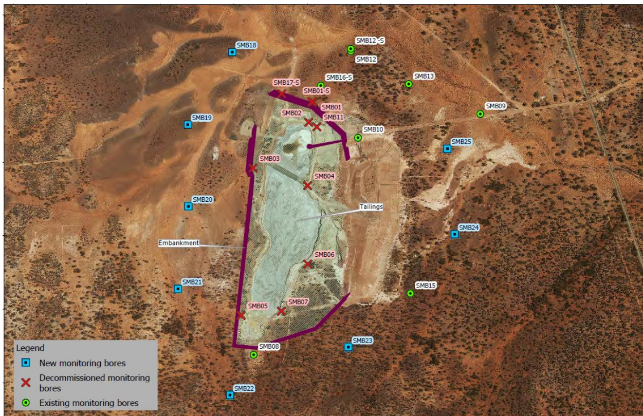
Figure 6: Saphire paddock style TSF – Monitoring network showing existing and proposed bores, including bores proposed to be decommissioned.
