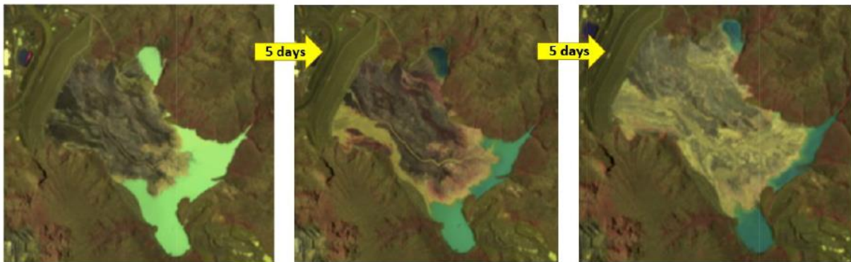
Figure 3 Sentinel Satellite imagery showing TSF1 water surfaces after a February 2020 storm
